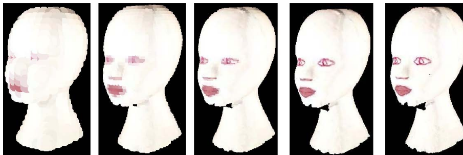
Figure 5.11: A multiresolution atlas supports progressive rendering. While a low resolution version is exhibited, high resolution models can be loaded in the GPU, avoiding delays in the change from editing to viewing mode.
